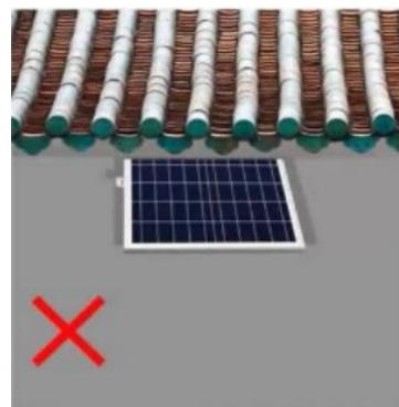
Solar panels cannot be installed in a place without or with less sunshine or will cause slow charging
